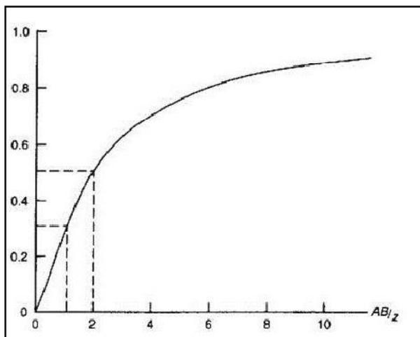
**Figure-6:** Fraction of current penetrating below a depth Z for a current electrode separation AB
