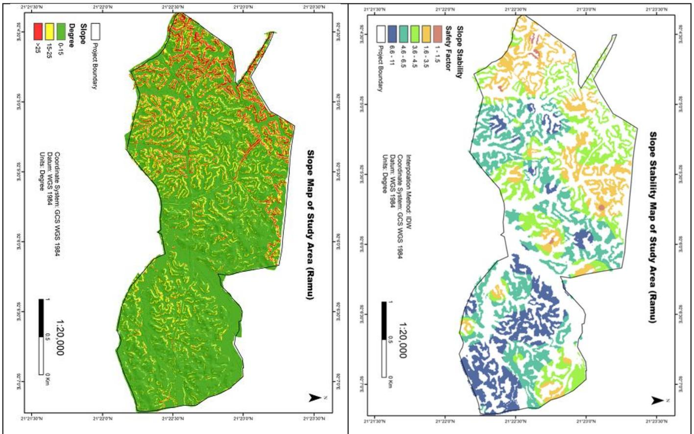
Figure 2.31 DEM based Slope Map and Slope Stability map
