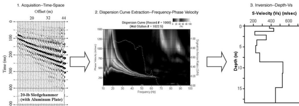
Figure 2.15 MASW data processing (Park et al., 1999)
