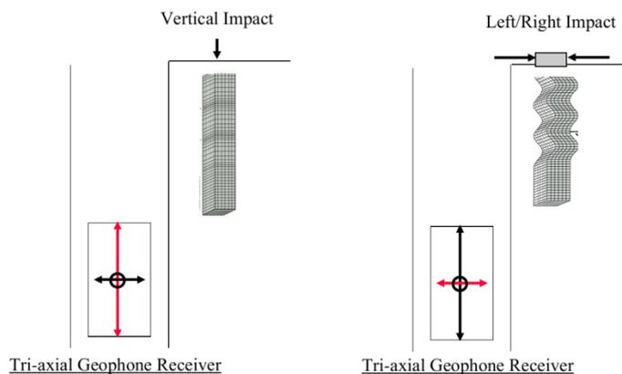
**Figure 2.11 Triaxial geophone behavior.**
