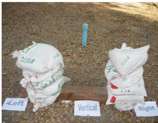
**Figure 2.10 Hit the wooden plank in 3 directions which are on the left, right and vertical directions.**
