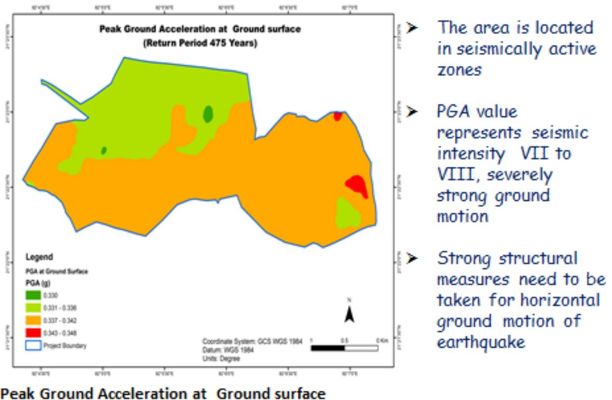
Figure 2.30 Seismic Hazard Map (Return Period 475 Years)
