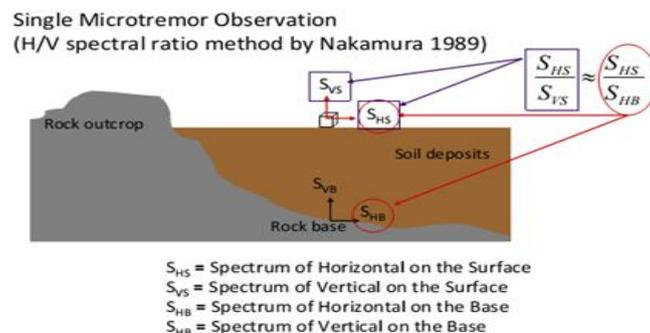
Figure 2.23 Fundamental of Single Microtremor observation
