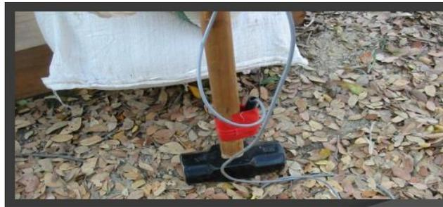
**Figure 2.6 To attach the trigger to a hammer.**
