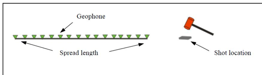
**Figure 2.17 Schematic of linear active source spread configuration**
