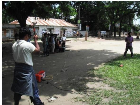
**Figure 2.18 MASW Field Data Acquisition**
