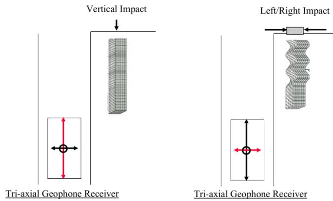
**Figure 2.11 Triaxial geophone behavior.**
