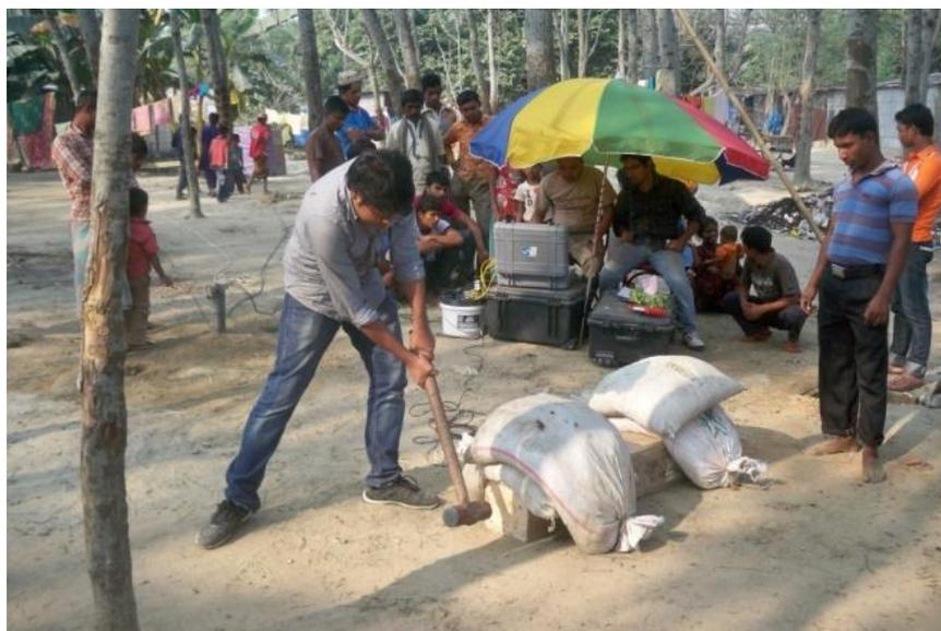
**Figure 2.1 Field Data Acquisition by PS logger**
