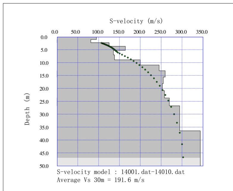
**Figure 2.22 One dimensional velocity structure for Passive MASW**
